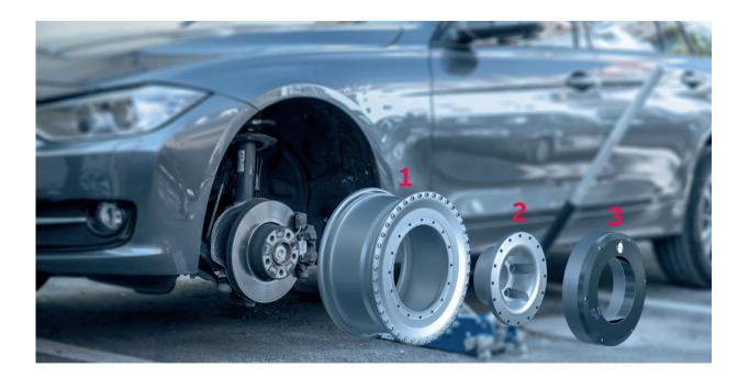
1 Rim adapter: As with a conventional rim, the rim adapter serves as a mount for the tire. The rim adapter is not directly specific to the vehicle, but depends on the tire. This allows it to be used on different vehicles with the same tire size.
