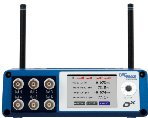
Fig. 2: The receiver unit (RCI) of the Dx telemetry system.
