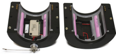
Fig. 3: Dx transmitter module (SCT) with integrated battery in a half-shell housing for mounting on drive shafts.
