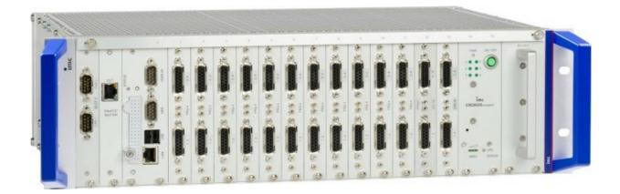
There are 16 free slots in a CRONOScompact AC- and DC-RACK. Your system can be freely configured with analog, digital and fieldbus modules. Exception #1: totally 16 analog or 16 digital modules, e.g. 16 analog and two digital modules. Exception #2: the SYNTH-8 294 module, this module will be detected as a fieldbus module.
