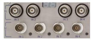
The connection is made via eight BNC sockets, four of which are for voltage measurement or optionally for ICP ( $\mathbf{U}$ ) and four for charge measurement ( $\mathbf{Q}$ ). The connections are labeled accordingly: U or Q
