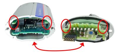
**Step 8:** Once the housing face is placed flush on the housing, the module can be closed tight with the Torx screws.
