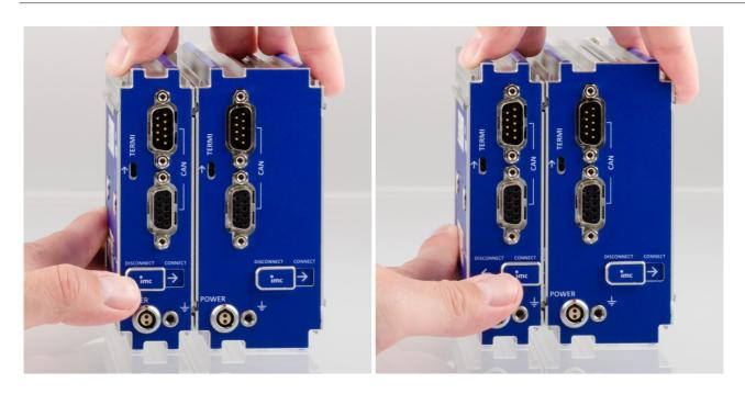
3. Slide the locking latch to the "CONNECT"-position.
