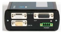
CANSS-IGN: CAN-connector and analog/digital outputs
