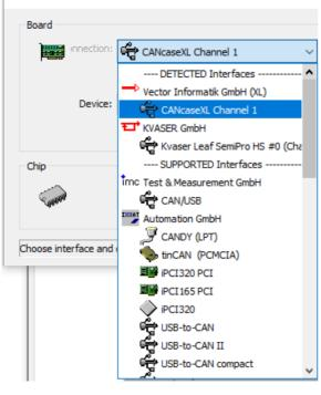
The interface cards supported by imc CANSAS are produced by many companies e.g. imc, KVASER, Vector, PEAK, XXAT and HORIBA. A selection of their installation software is located in the directory \*Driver*.
