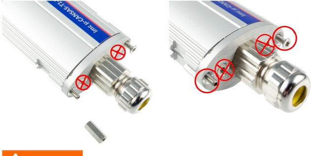
**Step 1:** Unfasten the grounding bolt and the **outer** Torx screw from the housing face.
