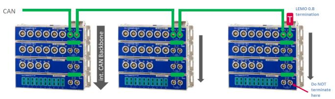
The CAN-Bus is only at the left most module active (side with the visible USB service connection):
