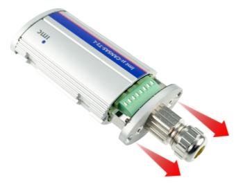
**Step 3:** Detach the connector junction with its Phoenix strip terminal from the housing face by gently bending the clamping brackets at the sides outward.
