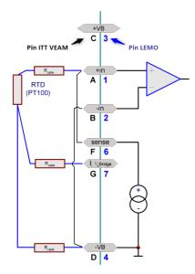
The PT100 is supplied with constant current via two lines (-SENSE and -VB). Another line (I, 1/4B) measures the voltage across the supply line and uses it to compensate for parasitic voltage drops. It is assumed that the resistances of the supply lines have the same size and the same temperature drift.
