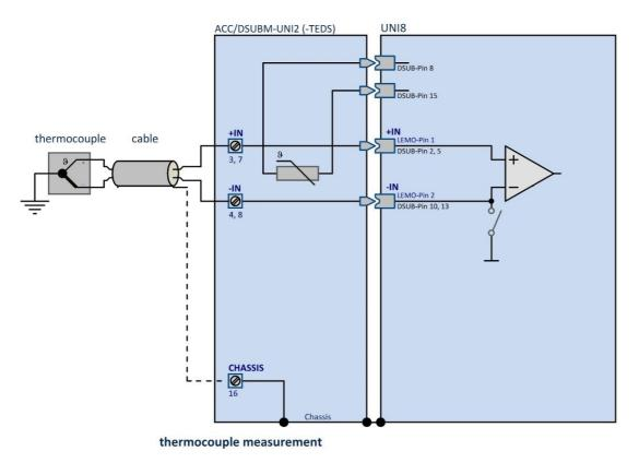
It is not a problem if the ground potential at the thermocouple differs from that of the device units by a few volts. However, the maximum allowed common mode voltage may not be exceeded.
