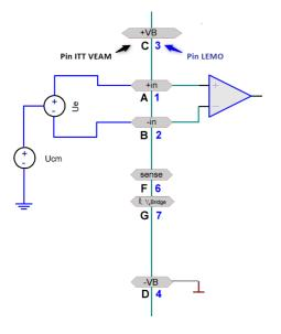
The common mode voltage ( $U_{cm}$ ) has to be less than ±10 V. It is reduced by  $\frac{1}{2}$  input voltage.
