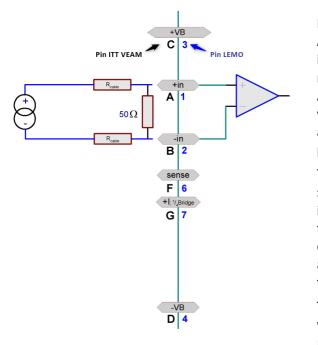
For current measurement could be used the DSUB plug ACC/DSUBM-I2. That plug comes with a 50  $\Omega$  shunt and is not included with the standard package. It is also possible to measure a voltage via an externally connected shunt. Appropriate scaling must be set in the user interface. The value 50  $\Omega$  is just a suggestion. The resistor needs an adequate level of precision. Pay attention to the shunt's power consumption.
