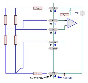
Please note that the maximum allowed voltage drop along a cable may not exceed approx. 0.5 V. This determines the maximum possible cable length.
