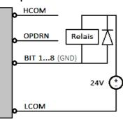
**Device off:** no continuity/high impedance  $(1.5 \text{ M}\Omega), 0 \text{ V}$  at output
