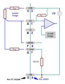
A quarter bridge can consist of a single strain gauge resistor, whose nominal value can be  $120 \Omega$  or  $350 \Omega$ .
