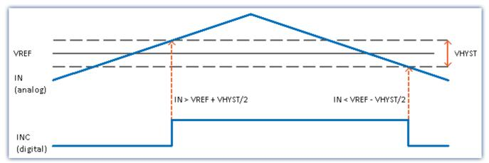
If the analog signal exceeds the threshold VREF + VHYST/2. the digital signal changes its state ( $\uparrow$ : 0  $\Rightarrow$  1) and at the same time reduces the threshold which must be crossed in order to change the state back to 0 by the amount VHYST (new threshold: VREF - VHYST/2). The magnitude of the hysteresis therefore represents the maximum level of noise and interference that would not cause a spurious transition.
