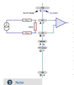
For current measurement the DSUB plug ACC/DSUBM-I2 is mandatory. The ACC/DSUBM-I2 comes with a 50  $\Omega$  shunt and is not included with the standard package. It is also possible to measure a voltage via an externally connected shunt. Appropriate scaling must be set in the user interface. The value 50  $\Omega$  is just a suggestion. The resistor needs an adequate level of precision. Pay attention to the shunt's power consumption.
