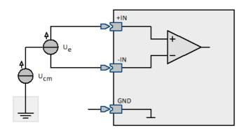
In the input ranges <20 V, the common mode voltage Ucm must lie within the range  $\pm 10$  V. It is reduced by one-half of the input voltage.
