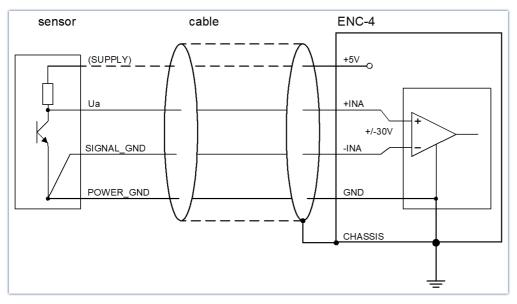
sensor with open-collector output
