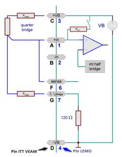
A half bridge may consist of two strain gauges in a circuit or a sensor internally configured as a half bridge, or a potentiometer sensor. The half bridge has 4 terminals to connect. For information on the effect and use of the SENSE lead, see the description of the <u>full bridge</u> 132.
