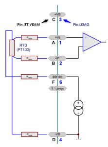
The PT100 is supplied with constant current via two lines (-SENSE and -VB). The other two serve as Sense-leads. By using the lines (+IN und -IN), the voltage at the resistor itself can be determined precisely. The voltage drop along the conducting cable thus does not cause any measurement error. The 4-wire configuration is the most precise way to measure with a PT100.
