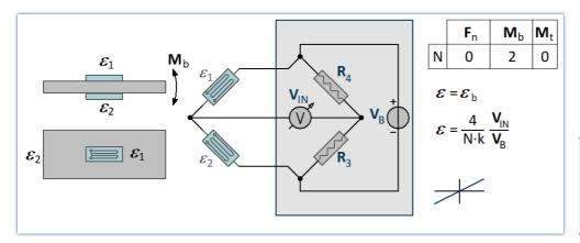
Longitudinal forces, torsion and temperature changes are compensated.
