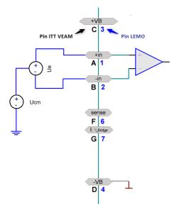
The common mode voltage ( $V_{cm}$ ) has to be less than ±10 V. It is reduced by ½ input voltage.
