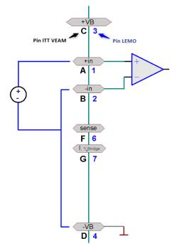
The voltage source itself is not referenced to the device ground but is instead isolated from it. In this case, a ground reference must be established. One way to do this is to ground the voltage source itself. Then it is possible to proceed as for "Voltage source with ground reference". Here, too, the measurement is differential. It is also possible to make a connection between the negative signal input and the device ground, in other words to connect -IN and -VB.
