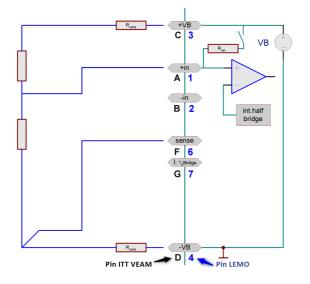
A half bridge may consist of two strain gauges in a circuit or a sensor internally configured as a half bridge, or a potentiometer sensor. The half bridge has four terminals to connect. For information on the effect and use of the Sense lead SENSE, see the description of the full bridge.
