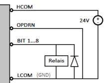
Device off: no continuity/high impedance (1.5 M $\Omega$ )
