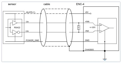
sensor with RS422 differential output
