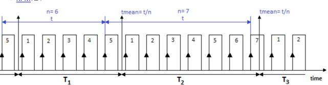
The frequency is determined as the number of events counted divided by the time between the first and the last "complete" event in the interval. An event is complete when a positive edge is succeeded by a subsequent positive edge.
