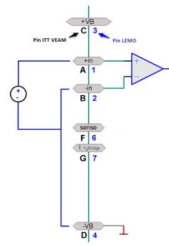
The voltage source itself is not referenced to the amplifier ground but is instead isolated from it. In this case, a ground reference must be established. One way to do this is to ground the voltage source itself. Then it is possible to proceed as for <u>Voltage source with ground</u> reference 130. Here, too, the measurement is differential. It is also possible to make a connection between the negative signal input and the device ground, in other words to connect -IN and -VB.
