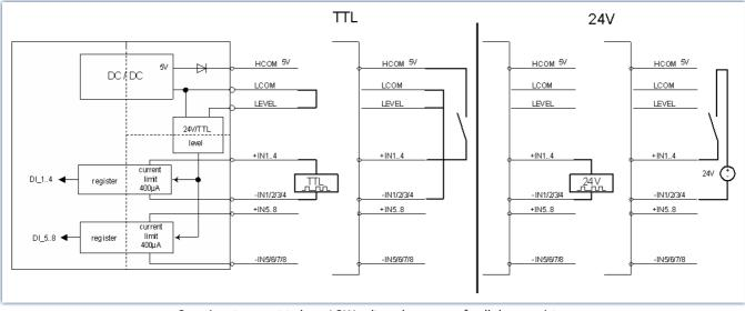
Open inputs are set to have LOW voltage by means of pull-down resistors
