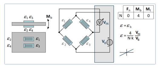
The sensitivity of the bending moment is increased. At the same time, longitudinal force, torque and temperature are compensated for.
