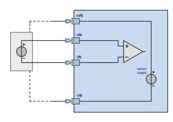
The sensor supply is unipolar and can be led out with DSUB-15 plugs at +VB and -VB (or +SUPPLY and -SUPPLY, see typing label in your plug). Only five selectable settings are available per module. The configurations can be taken from the respective module data sheet. The voltage can be set globally for all channels of a module. All channels of a module form a channel group.
