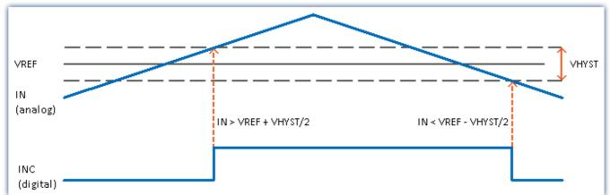
The *digital signal* changes from **0 to 1** when the *analog signal* exceeds the **VREF + VHYST/2** threshold.
