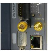
WiFi - antenna with SMA (male) connection at your device SMA (female)
