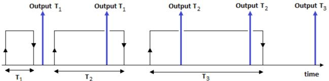
Above is illustrated a measured signal from which time readings are taken. Each reading starts at a positive edge in the signal and is stopped at a negative edge. The "up" arrows indicate the times at which the system returns a result. The returned values in this case are T1 –twice; T2 –twice; and T3.
