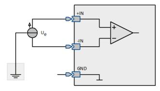
The voltage source itself already is referenced to the device's ground. The voltage source is at the same potential as the device ground.
