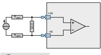
In this configuration, too, the maximum common mode voltage must be located within the range: ±10 V. This can generally only be assured if the current source is also already referenced to ground.
