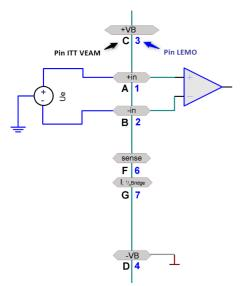
The voltage source itself already has a connection to the device's ground. The potential difference between the voltage source and the device ground must be fixed.
