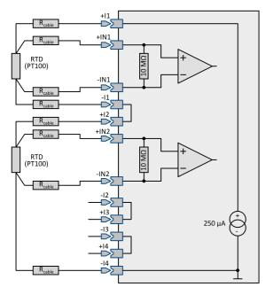
Along with thermocouples, **PT100** sensors can also be connected, in **4-wire configuration**. An extra reference current source feeds an entire chain of up to four serially connected sensors.
