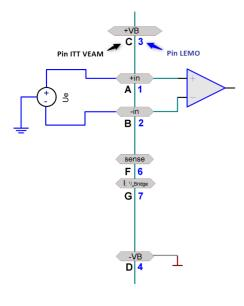
The voltage source itself already has a connection to the device's ground. The potential difference between the voltage source and the device ground must be fixed.
