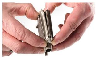
ACC/DSUBM-xxx: snap the nose into the slot
