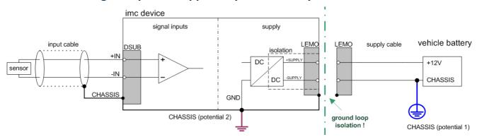
imc CL Devices with isolated DC-supply (e.g. battery)
