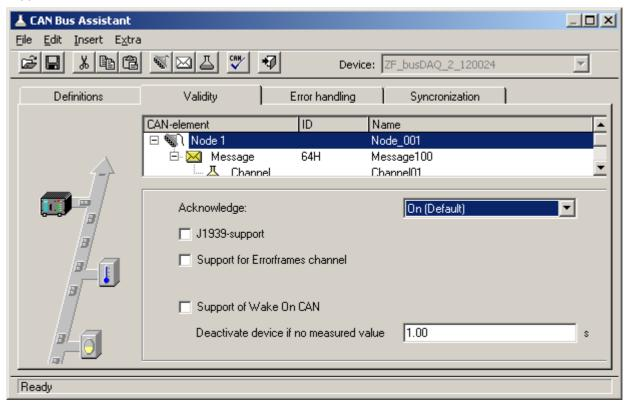
The option Support of *Wake On CAN* appears on the page Validity if a node is selected in the CANelement tree diagram. If it isn't shown, this indicates that your device's hardware isn't set up for this function.
