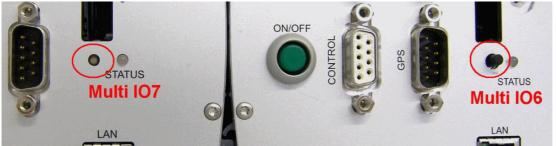
From Multi IO7 onwards, the button is countersunk, so that to press it a sharp object like a pen is needed. Up until Multi IO6 the button was black and protruding.
