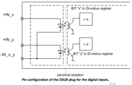
Pinconfiguration of the DSUB15 plugs for the digital inputs 51.
